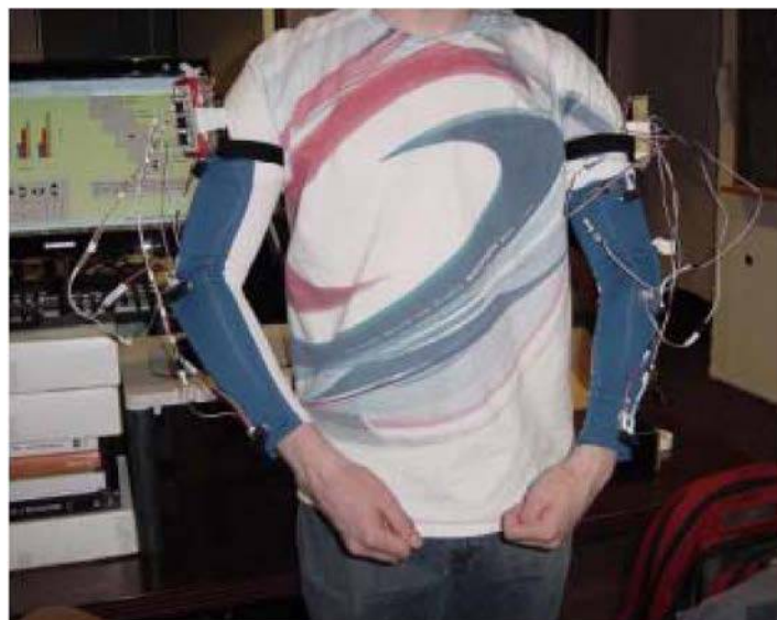
Plate 1 Early prototype for the arm sensor-vibrotactile set; two sets on two arms, each having three pairs of sensors
