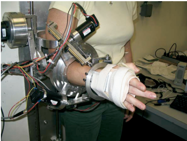
Fig 3. A robotic lower-arm exoskeleton provides sensing and actuation for elbow flexion and extension, wrist pronation and supination, and radial-ulnar deviation. 52
